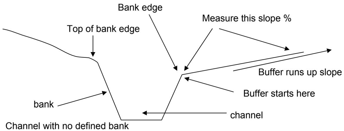
Measure slope % from center of drainage channel, use 2 feet for every % slope to set buffer width. Buffer must be made up of at least 25 feet forest and 20 feet filter strip. The forest portion must be along the drainage channel.
